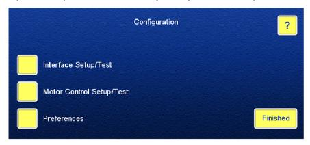
The Interface Setup/Test was moved from the System page, and contains the main machine model selection and stitching control settings.
