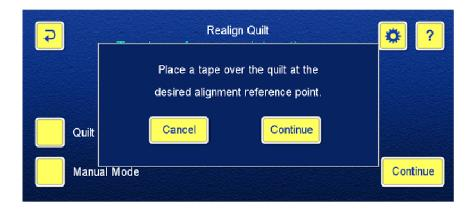
As the next step, you move the needle over the tape. Remember to take the thread out of the needle, for the iQ will take a single stitch in the tape when you touch [Continue].
