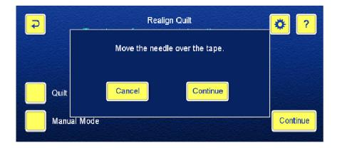
Now you are asked to advance the quilt. You need to ensure that the needle hole in the tape remains reachable. The motors are lifted at this point, so you can baste down the edges, if that is your preference.
