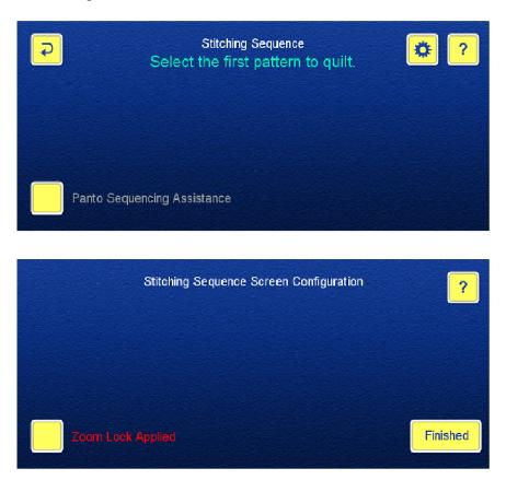
Panto Sequencing Assistance is a new feature that has been added to the Stitching Sequence page. This feature lets you sequence several rows of a pantograph by setting up the rules that will be repeated either step by step, or throughout the whole quilt. The Panto Sequencing Assistance button is enabled when at least one row is selected manually. When you touch the button, the following pop-up messages guide you through the auto sequencing process.
