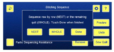
The **Required quilting depth** display will help you determine how many rows can be sequenced. The displayed number is the distance between the highest point of the pattern at the top and the lowest point of the pattern at the bottom of the sequence. Compare this number to the quilting space you have between the bars, after taking the rolled-up quilt into consideration.
