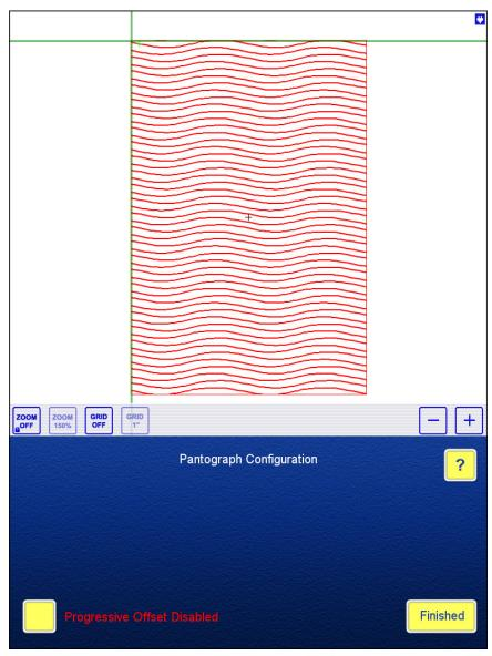
But when you enable the progressive offset, this is the resulting pattern. The progressive offset can create interesting effects using otherwise simple pantograph patterns. We hope that this unique feature of the iQ will inspire pattern designers to create patterns that are specifically suited for progressive offset.
