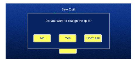
The **Adjust Before Start** option was added to the local configuration of the Sew Quilt screen. When this option is enabled, the program goes to the Adjust page, without moving the needle to the start point. When the adjustment is finished, the needle will move to the new starting point.
